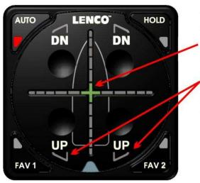
WHEN YOUR BOAT'S <u>CURRENT</u> <u>ROLL AND PITCH POSITIONS</u> MATCH THE AUTO GLIDE'S <u>HOME ROLL AND</u> <u>PITCH DEFAULT POSITIONS</u>, ONLY THE GREEN CENTER LED IS ILLUMINATED ON THE CROSSHAIR LED INDICATORS.
