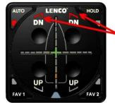
DURING AN AUTOMATIC BOAT CONTROL DECISION, THE AUTO GLIDE EXTENDS BOTH ACTUATORS TO CORRECT FOR A PITCH ANGLE THAT IS ABOVE THE HOME PITCH POSITION.
