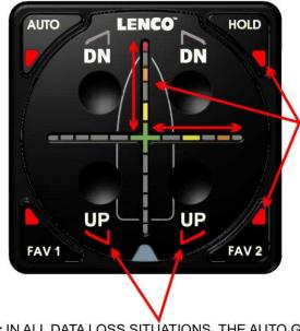
WHEN ENGINE DATA LOSS OCCURS, THE AUTO GLIDE WILL FLASH THE OUTSIDE FOUR (4) <u>AUTOMATIC</u> <u>SETTING LED INDICATORS</u> AND THE CROSSHAIR LED INDICATORS WILL SCROLL FROM THE <u>CENTER</u> <u>TO THE TWELVE O'CLOCK</u> POSITION AND FROM THE <u>CENTER TO THE</u> THREE O'CLOCK POSITION.
