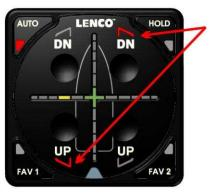
TO MAKE A ROLL CORRECTION, THE AUTO GLIDE MOVES BOTH THE PORT AND STARBOARD TRIM TABS AT THE SAME AMOUNT, BUT IN THE OPPOSITE DIRECTION.
