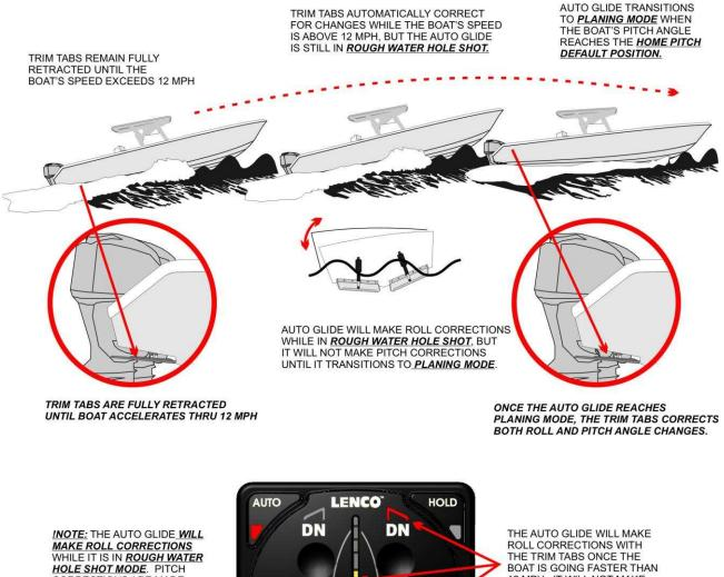
MAKE ROLL CORRECTIONS WHILE IT IS IN ROUGH WATER HOLE SHOT MODE. PITCH CORRECTIONS ARE MADE ONCE THE AUTO GLIDE TRANSITIONS TO PLANING MODE.
