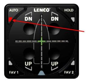
PRESS WHICHEVER OF THE FOUR (4) AUTOMATIC SETTING BUTTONS (IN THIS EXAMPLE YOU PRESS THE AUTO BUTTON) AND THE AUTO GLIDE WILL OVERRIDE IDLE MODE AND TRANSITION DIRECTLY INTO HOLE SHOT MODE.
