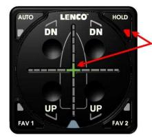
ONCE THE AUTO GLIDE HAS SAVED THE ALTERNATIVE HOME ROLL AND PITCH POSITIONS FOR <u>"HOLD"</u>, THE LED INDICATOR WILL ILLUMINATE.
