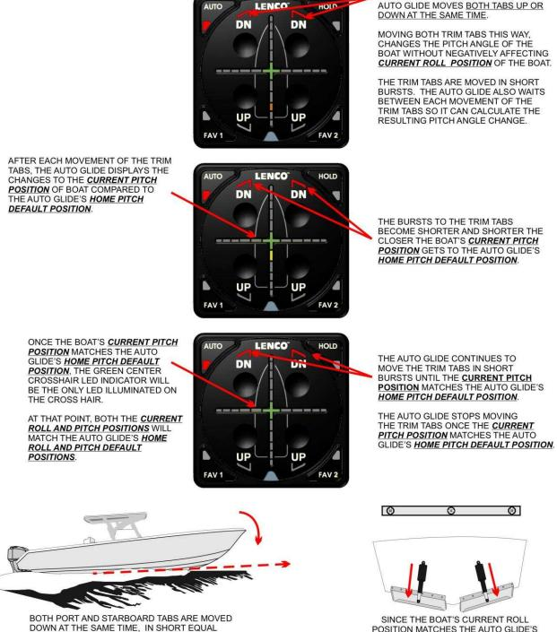
Down at the same time, in short equal Bursts until the boat's <u>current pitch</u> <u>Position</u> matches the auto glide's <u>home</u> <u>Default Pitch Position</u>. POSITION MATCHES THE AUTO GLIDE'S HOME ROLL DEFAULT POSITION, NO ROLL CORRECTIONS ARE REQUIRED.
