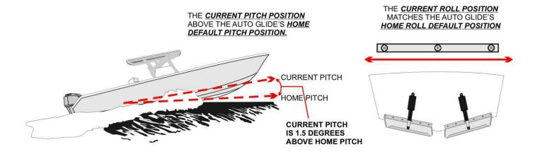
THE 3RD LED ON THE BOTTOM HALF OF THE VERTICAL CROSSHAIR LED INDICATOR IS ILLUMINATED TO INDICATE THAT THE BOAT'S **CURRENT PITCH POSITION** IS ABOVE THE AUTO GLIDE'S <u>HOME PITCH</u> **DEFAULT POSITION**.
