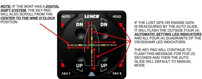
IF THE LOST GPS OR ENGINE DATA IS REACQUIRED BY THE AUTO GLIDE, IT WILL FLASH THE OUTSIDE FOUR (4) AUTOMATIC SETTING LED INDICATORS
