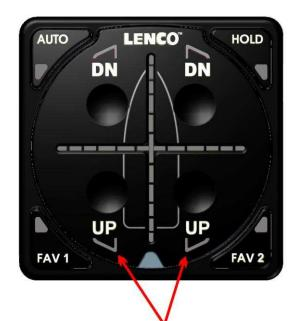
IF THE KEY PAD LOSES COMMUNICATION WITH THE AUTO GLIDE CONTROL BOX, THE KEY PAD WILL GO BLANK AND NO LED INDICATORS WILL BE ILLUMINATED.
