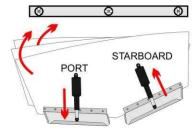
THE STARBOARD TRIM TAB IS MOVED UP AND THE PORT TRIM TAB IS MOVED DOWN IN SHORT, EQUAL BURSTS UNTIL THE BOAT'S CURRENT ROLL POSITION MATCHES THE AUTO GLIDE'S HOME ROLL DEFAULT POSITION
