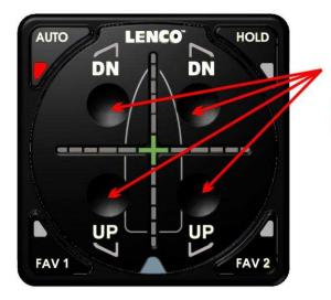
PRESS ANY OF THE FOUR (4) UP/DN BUTTONS TO ACTIVATE MANUAL MODE.
