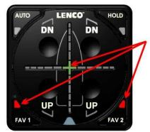
ONCE THE AUTO GLIDE HAS SAVED THE ALTERNATIVE HOME ROLL AND PITCH POSITIONS FOR "FAV 1" OR "FAV 2", THE CORRESPONDING LED INDICATOR WILL FLASH FIVE (5) TIMES.
