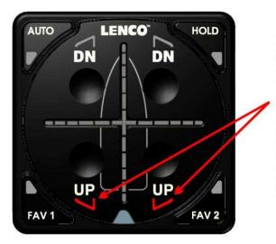
BOTH <u>UP ACTUATOR LED</u> <u>INDICATORS</u> FLASH AS THE AUTO GLIDE RETRACTS THE TRIM TAB ACTUATORS TO ENSURE THE TRIM TABS ARE FULLY RETRACTED.
